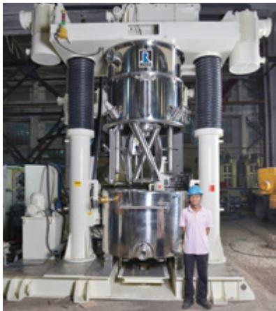
apply intense shear to achieve a smooth, uniform consistency. The PDDM is rated for vacuum operation up to 29.5 in. Hg and includes a jacketed change-can vessel, sight/charge ports on the cover and an automated lift for raising and lowering the agitators.
