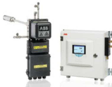
The sensor assembly mounts to a duct or process wall, with the probe extending into the flue gas stream. Available in lengths up to 8+ ft (2.5 m) and suitable for temperatures to 3,000°F (1,650°C), the probe continuously draws in the sample for analysis.
